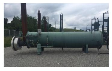
Water reduction to <7 lbs./Mft<sup>3</sup> will allow for depression of hydrate formation temperature and control system corrosion by limiting water interaction with H<sub>2</sub>S and CO<sub>2</sub> gases.
